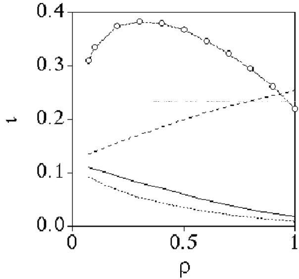
**Fig. 2.** Radial variation of the vacuum rotational transform (solid curve) and its external (dashed) and internal (dotted) components. The total rotational transform for the case with strong bootstrap current is shown by the curve with circles.
