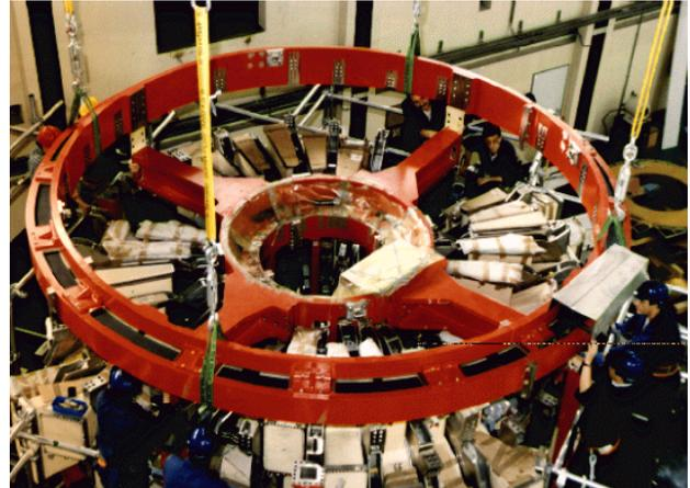
**Fig. 2.** The picture shows the moment when the outer ring of the support structure holding the vertical field coil was placed in position, completing the coil assembly.
