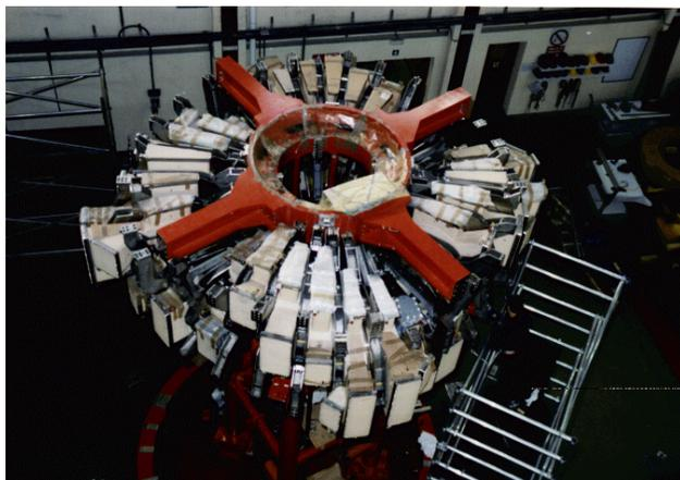
**Fig. 1.** The helical structure of the TJ-II vacuum chamber can be appreciated in the distribution of the 96 experimental ports
